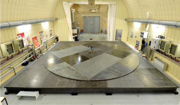
Fig. 12: Large iron shielding above the detector.
