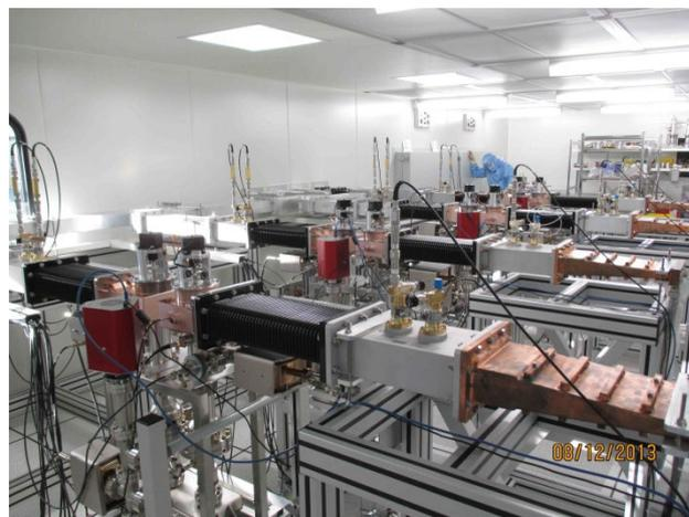
Figure 10: European XFEL High Power Coupler test stands at LAL, Orsay, consisting of four RF power lines (shown here), each populated with two HPCs located in an ISO4 clean room.
