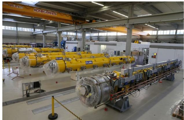
Figure 12: Cryo-modules in the test hall AMTF. In the foreground a fully equipped Cryo-module with the tailored wave guide distribution system attached ready for tunnel installation. The test stand shielding is visible in the background.
