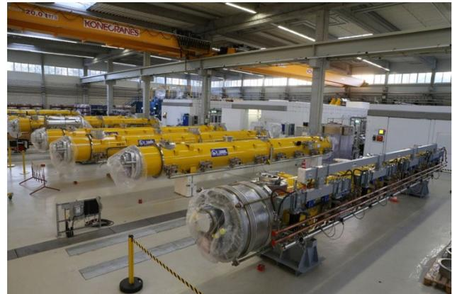
Figure 12: Cryo-modules in the test hall AMTF. In the foreground a fully equipped Cryo-module with the tailored wave guide distribution system attached ready for tunnel installation. The test stand shielding is visible in the background.
